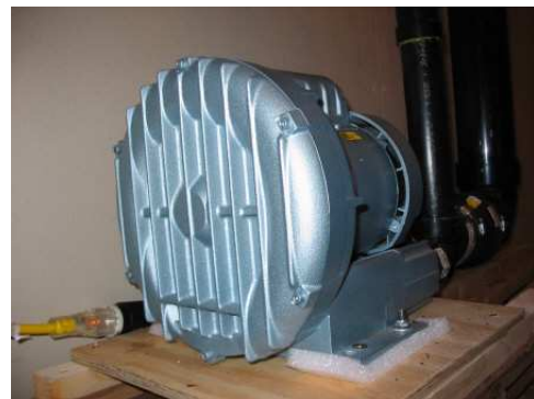
Figure 3. The GAST R6 blower used to supply fresh air to the containers. This low pressure blower supplies approximately 80 L/min. to each container.
