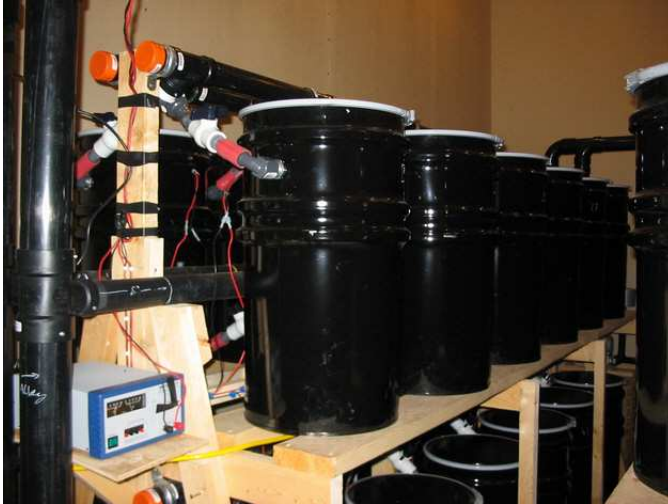
Figure 1. General view of the setup of the treatment chambers showing the ventilation system, the adjustable voltage power supply, and some of the 63 liter containers.
