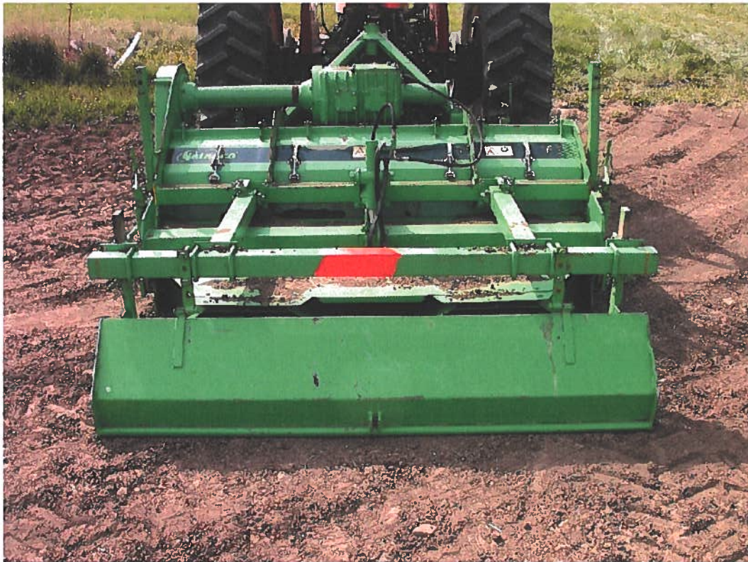
Fig. 2. Power-hiller set to form 1.8 m wide bed.
