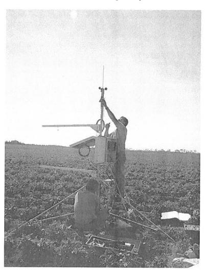
Figure 1. Initial installation of BREB system.
