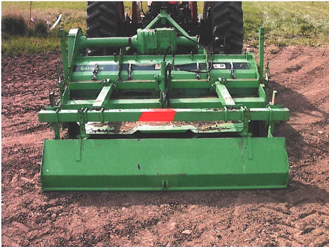
Fig. 2. Power-hiller set to form 1.8 m wide bed.
